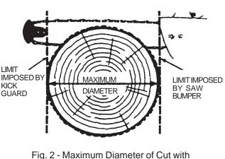
Fig. 2 - Maximum Diameter of Cut with Kick Guard Installed
